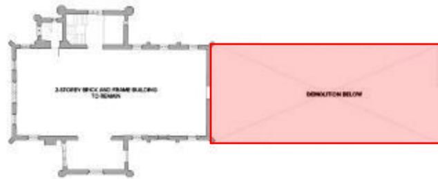
Second level demolition plan
